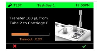
**Use the SAME pipette** to slowly transfer 100 μL from Tube 2 to Cartridge Tube B.
