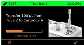
**Use the second pipette** provided to slowly transfer 100 µL from Tube 2 to Cartridge Tube A
