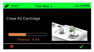
Fold the cartridge lid over and press down firmly to cap the cartridge. **Ensure an audible click is heard.**
