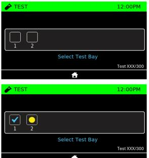
Select an "Empty" test bay to start a test in that bay.
