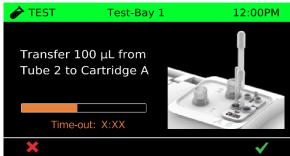
**Use the second pipette** provided to slowly transfer 100 µL from Tube 2 to Cartridge Tube A
