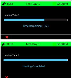
Wait 2 minutes for the instrument to heat Tube 1 by allowing the timer to elapse on the screen.
