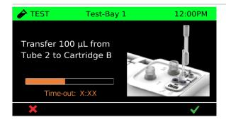
**Use the SAME pipette** to slowly transfer 100 μL from Tube 2 to Cartridge Tube B.
