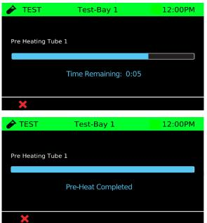
Wait 20 seconds for the instrument to pre-heat Tube 1 by allowing the timer to elapse on the screen. A double beep will sound when the Pre-Heating time is complete.
