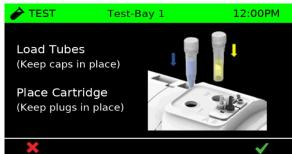
Tear open the **ZiP-CoVx-P2 Buffer Pack**. Place the sample preparation tray on the instrument deck. Insert Tube 1 (blue) into the "1" hole and Tube 2 (yellow) into the "2" hole. Ensure tubes are seated all the way down. Leave the pipettes in the buffer pack until use.
