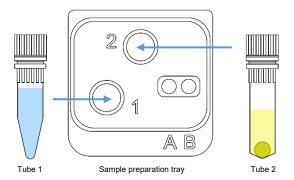
Tear open the **ZiP-CoVx-P2 Cartridge Pack**. Insert the P2 cartridge into the "A" and "B" holes on the sample preparation deck. Ensure the barcode is facing you.
