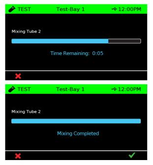
Wait for Tube 2 Mixing to complete by allowing the timer to elapse as shown on the screen. A double beep will sound when mixing is complete.
