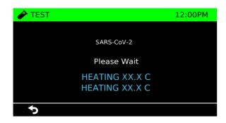
Wait for the heater blocks to reach the pre-set test type temperature. This screen will not show if the heater blocks are already at temperature.
